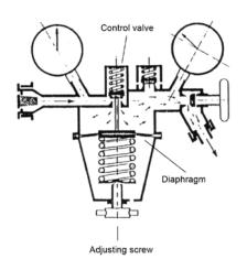
**Note:** New standards governing the condition and testing of pressure reducers came into force in the mid-1990s (DIN EN ISO 2503, DIN EN 961, 738-1, 738-2). In accordance with these standards, adjustable oxygen pressure reducers must successfully complete a burn-out test with pressure surges both with the control valve closed as well as with the control valve opened.
