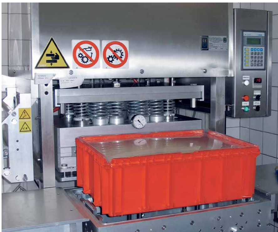
Creation of a protective atmosphere in reusable containers
