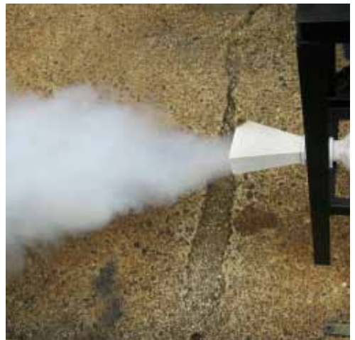
Figure 14: Special nozzle for vaporising carbon dioxide [4]
