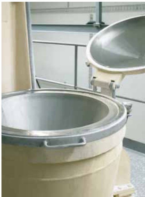
Figure 17: Inert gas sluice (shown here: N 2 LOCK™ from Linde)
